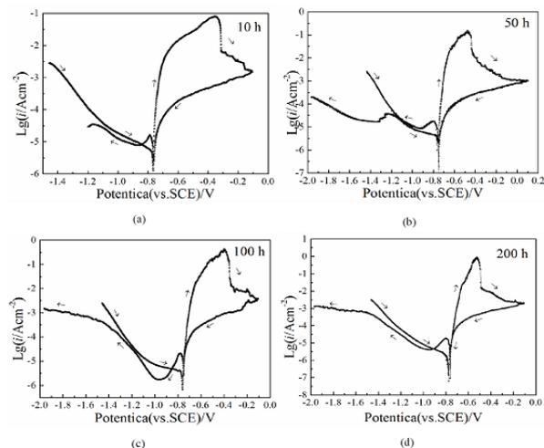
**Figure 4:** Polarization curves of the oxide films grown on as-spun Al86Ce10Ni4 at 630°C in static air for (a) 10, (b) 50, (c) 100, and (d) 200 hours.
