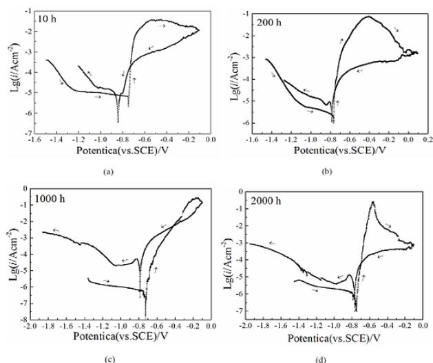
**Figure 3:** Polarization curves of the oxide films grown on as-spun Al86Ce10Fe4 at 630 °C in static air for (a) 10, (b) 200, (c) 1000, and (d) 2000 hours.
