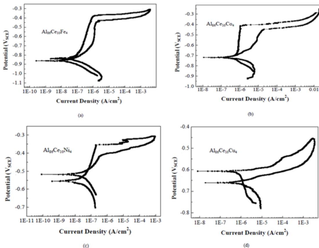
**Figure 1:** Electrochemical polarizations of the as-spun amorphous Al<sub>86</sub>Ce<sub>10</sub>TM<sub>4</sub> (TM= Fe (a), Co (b), Ni (c), and Cu (d) alloys in 3.56 wt.% NaCl solution.
