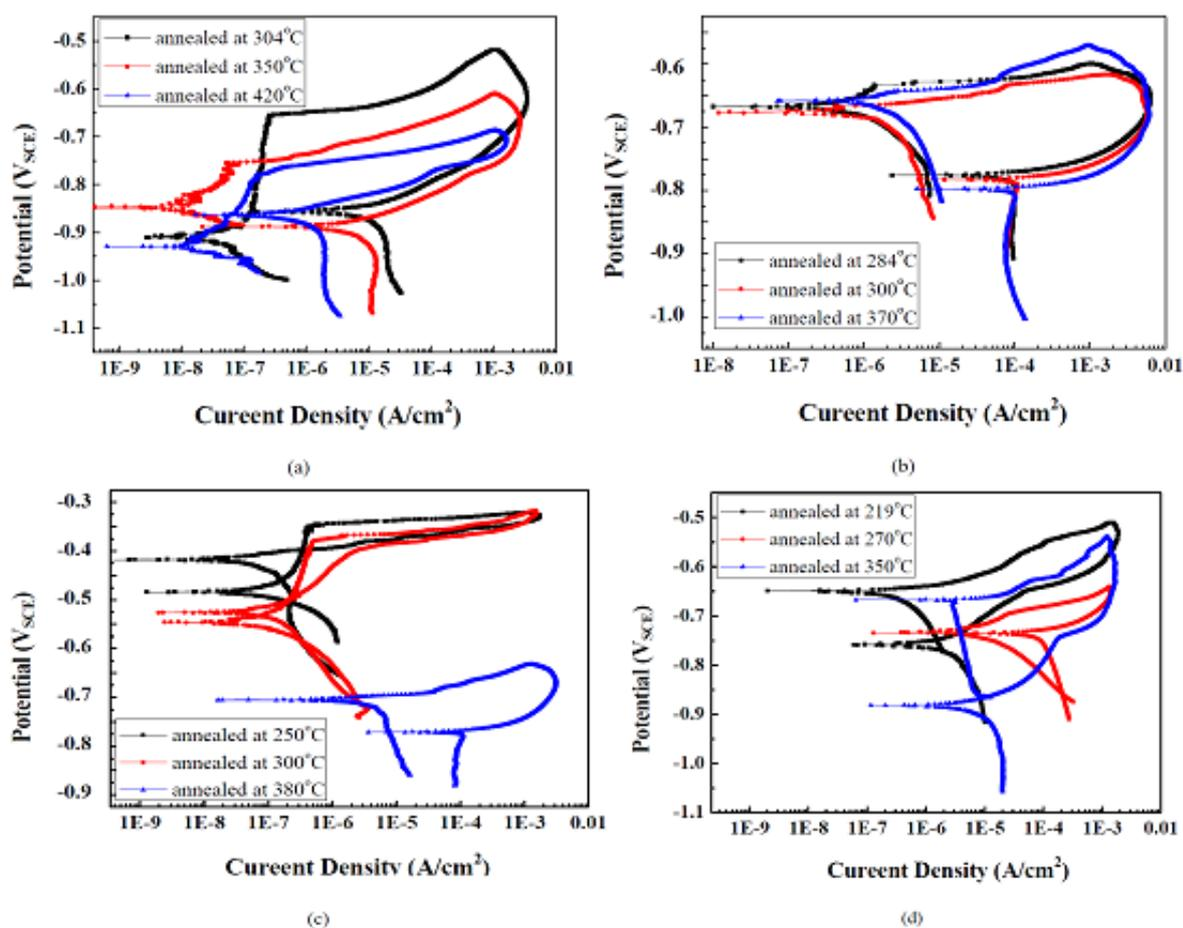
**Figure 2:** Electrochemical polarizations of the post-annealed Al<sub>86</sub>Ce<sub>10</sub>TM<sub>4</sub> (TM=Fe (a), Co (b), Ni (c) and Cu (d)) alloys in 3.56 wt. % NaCl solution.
